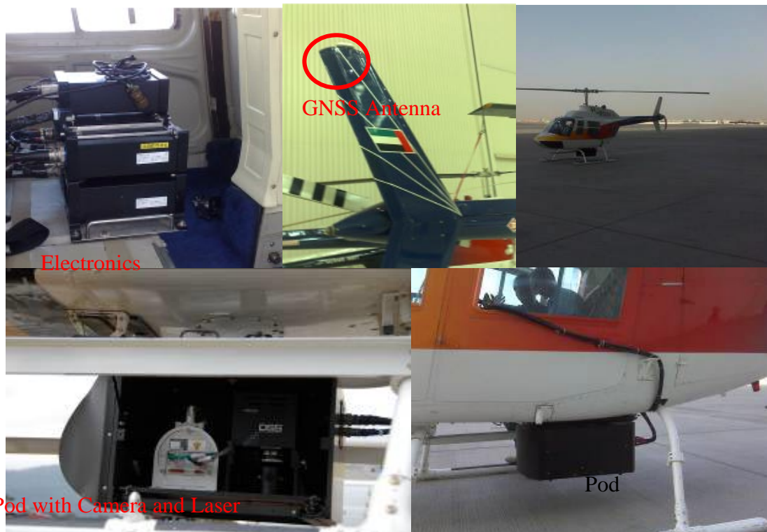
Figure 4: The airborne System mounted in Bell 206.
