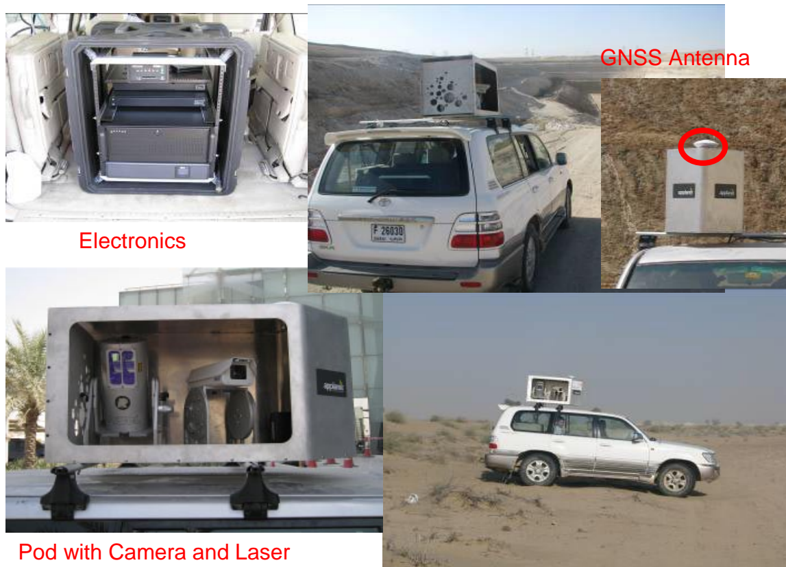
Figure 5: The Land Mark System mounted on Land cruiser car.
