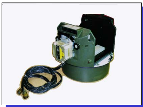
Figure 11: IMU Mounted in Handle of RC30 Camera
